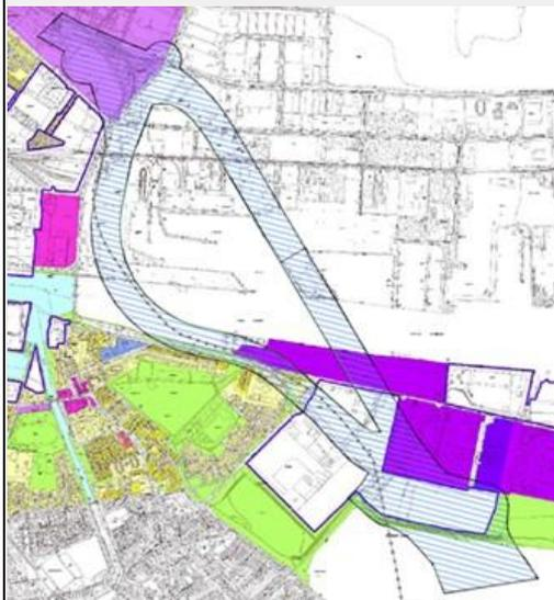
**2009:** NRA progressed a Corridor Protection Study for Sector A of the DEB, which protected these two corridors (as indicated in the image extracted from the report). The corridor to the west was for a cut & cover tunnel, and the corridor to the east for a high-level skew bridge.
